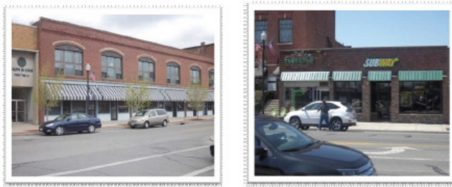
Figure 20: Encouraged Awnings- Awnings that are to scale with the windows and entry of the building.
